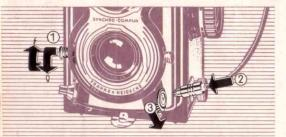
Choice of Contact: Pull knob ① and set on \$\foatstyle{\psi}\$ for electronic flash (≯ page 26); this X-contact is also automatically used with self-timer shots (≯ page 27) — set on ② when using M-type flash bulbs (≯ page 26).
