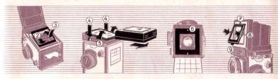
Inserting the Film Mask: Insert the spring loaded side behind the film aperture frame (3), first below (2), then above.
